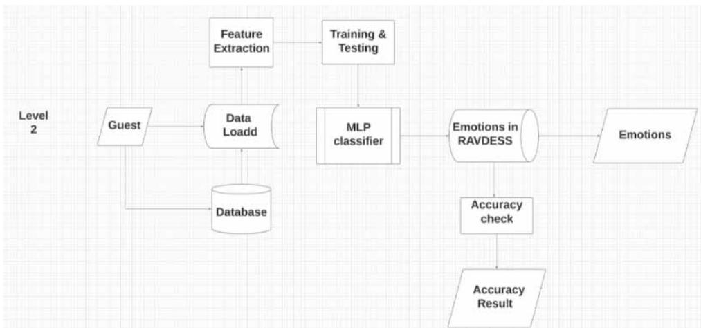
Figure 15. User case diagram for extraction emotion from user speech
